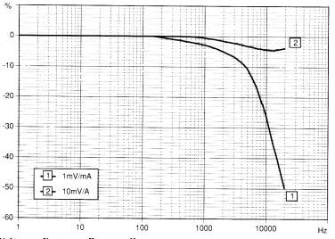
Voltage vs Frequency Response Curve
